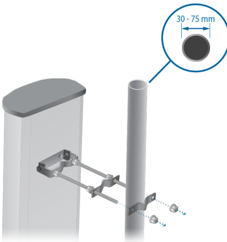
Figure 8: Pole mounting. Source: AM-9M13 Quick Start Guide ([www.ui.com/airmax/airmax-sector-antenna/](http://www.ui.com/airmax/airmax-sector-antenna/))
