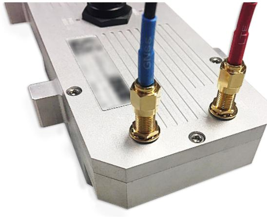
Figure 5: GPS and LTE Antenna cable plug
