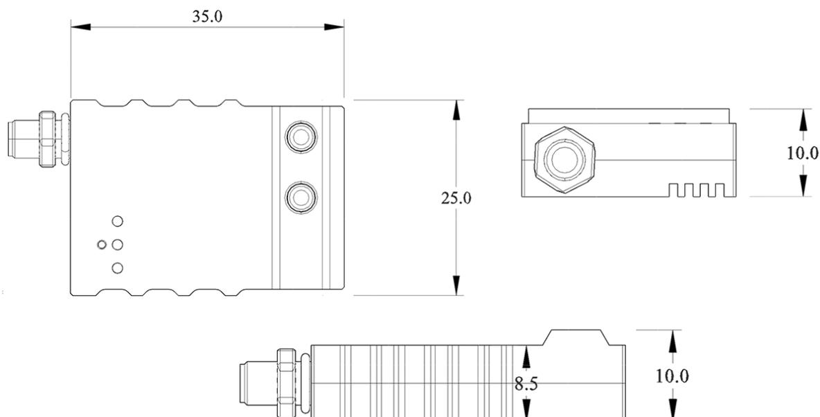
Figure 2: Dimensions of Transceiver TR-1A
