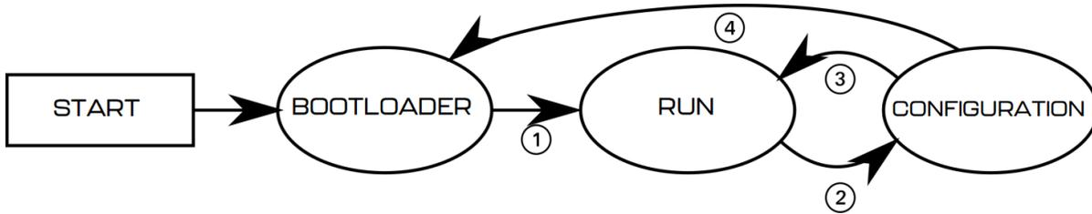
Figure 3: State machine of Transceiver TR-1A
