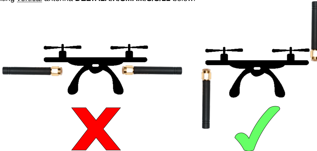
Figure 5: Proper antennas mount
